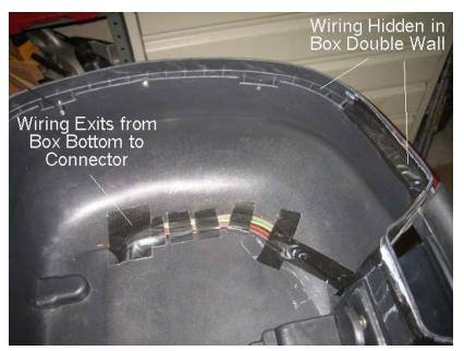
Here you can see that the strip wiring (including diodes and resistors) has been pushed down into the double wall void, and covered with gaffer's tape. The male connector wires have been run through a hole drilled in the front bottom of the box, spliced to the wires from the strips, and then secured to the interior of the box with tape.
