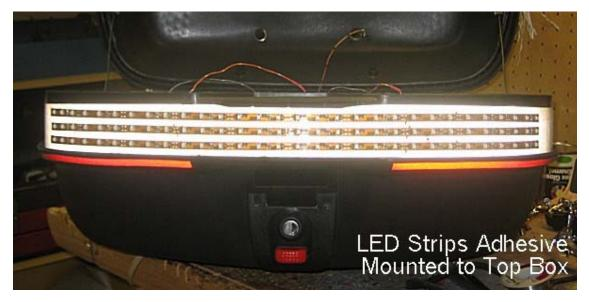
**Wiring:** The LED strips do not draw much current (~160mA for 30 LED Strip) so very small wires will suffice. I actually used conductors salvaged from an old multiconductor telephone cable inside the box – probably 26 or 28 gauge. Basically most all of the wiring and electrical components will wind up in between the double walls of the box behind the LED strips. Each strip will require only one pair of leads, positive and negative. The circuit is as follows:
